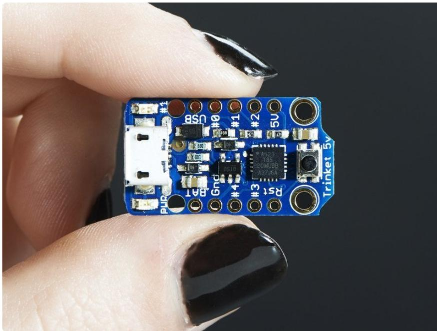
Trinket may be small, but do not be fooled by its size! It's a tiny microcontroller board, built around the Atmel ATTiny85, a little chip with a lot of power. We wanted to design a microcontroller board that was small enough to fit into any project, and low cost enough to use without hesitation. Perfect for when you don't want to give up your expensive dev-board and you aren't willing to take apart the project you worked so hard to design. It's our lowest-cost arduino-IDE programmable board!
