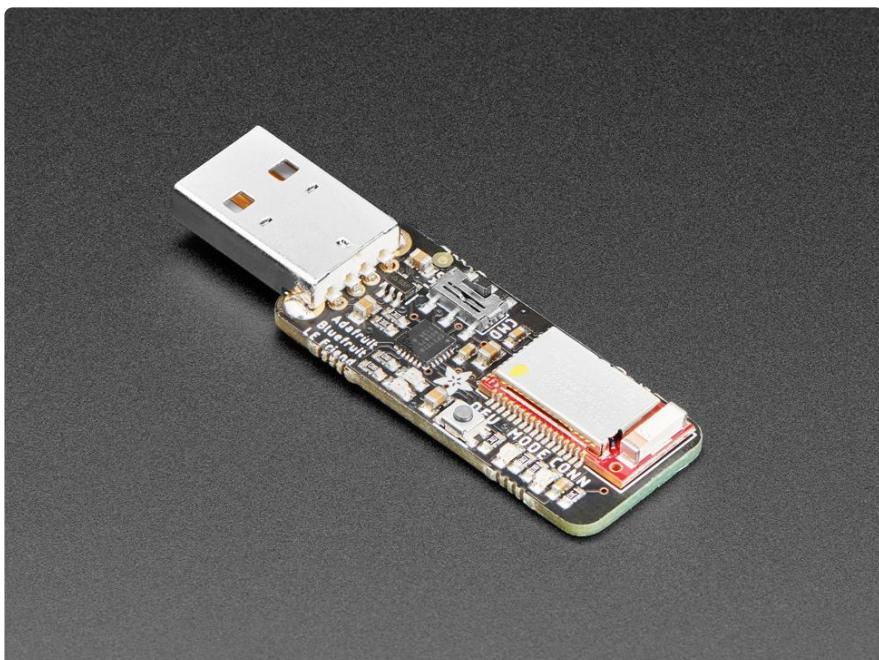
In its simplest form, it works on the same principle as a common USB/Serial adapter (the [FTDI Friend](http://adafru.it/284) (<http://adafru.it/284>), for example!). Any data that you enter via your favorite terminal emulator on your development machine will be transferred over the air to the connected phone or tablet, and vice versa.
