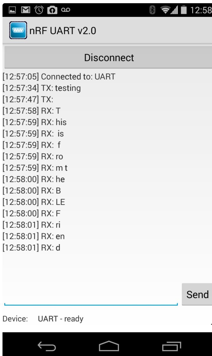
The incoming data is broken up into small packets because it is transferred in chunks of up to 20 bytes per payload.
