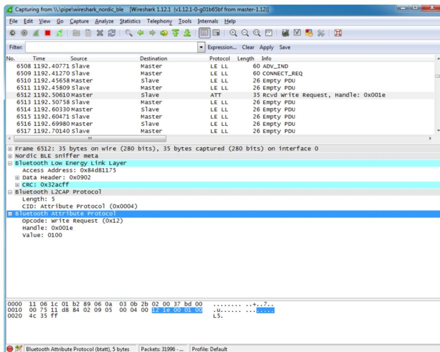
What this write request is trying to do is enable the 'notify' bit on the [UART service's TX characteristic \(https://adafruit.it/iCn\)](#) (0x001E is the handle for the CCCD or '[Client Characteristic Configuration Descriptor \(https://adafruit.it/ecl\)](#)'). This bit enables an 'interrupt' of sorts to tell the BLEFriend that we want to be alerted every time there is new data available on the characteristic that transmits data from the BLEFriend to the phone or tablet.
