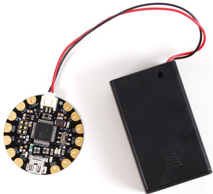
After loading your program onto the FLORA, you'll want to unplug the USB cable and go portable with battery power! USB will always power the board, but battery power (through the JST connector) can be turned on and off with Flora's onboard switch (near the "ON" text on the board). We recommend our [3xAAA holder](http://adafru.it/727) (<http://adafru.it/727>) for beginners, which conveniently plugs into FLORAs JST port.
