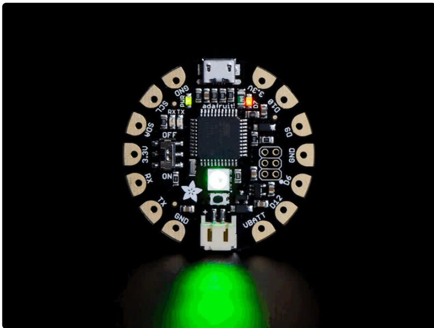
FLORA is Adafruit's wearable electronics platform. We designed it from the ground up to provide the best experience for Adafruit's community of makers, hackers, crafters, artists, designers and engineers. It's built around the Atmega32u4 chip, which has built-in USB support. No pesky special cables or extra parts for programming, just plug it in and get started making the wearables project of your dreams! Works on Windows and Mac.
