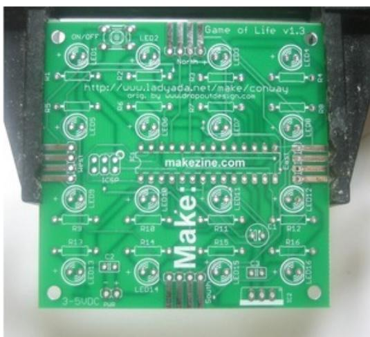
Take the PCB and place it in a vise or other holder so that you can easily place and solder parts.
