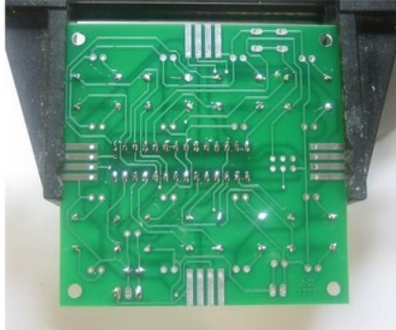
The socket has short legs so it's more likely to slip than a resistor. The easiest way to solder the socket is to hold it against the PCB with one finger (or tape) then solder in two points on opposite sides. Once you've got it tacked, solder in the remaining pins.
