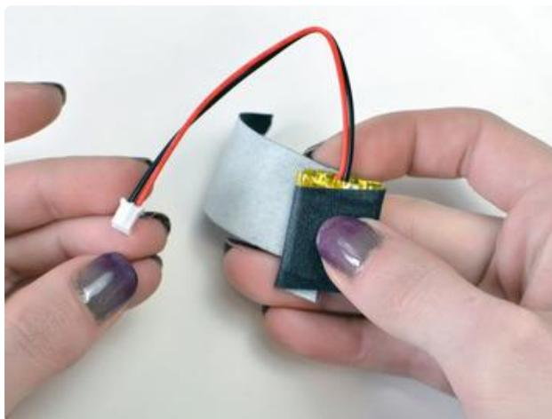
Tape up the battery to protect it and protect the wire connections.
