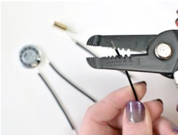
Use wire strippers to strip the insulation off the last quarter inch of each end of each wire.
