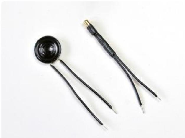
Your speaker and tilt ball switch are now ready for attaching to the rest of your circuit!
