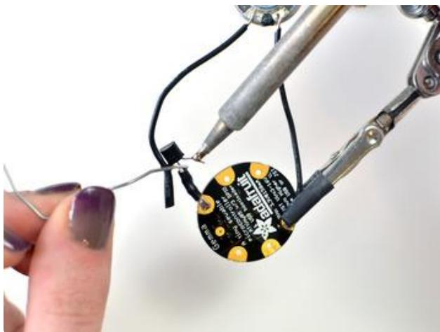
Tin the last remaining lead of the transistor and solder to a piece of wire. Slide on some heat shrink and use a heat gun to shrink it.
