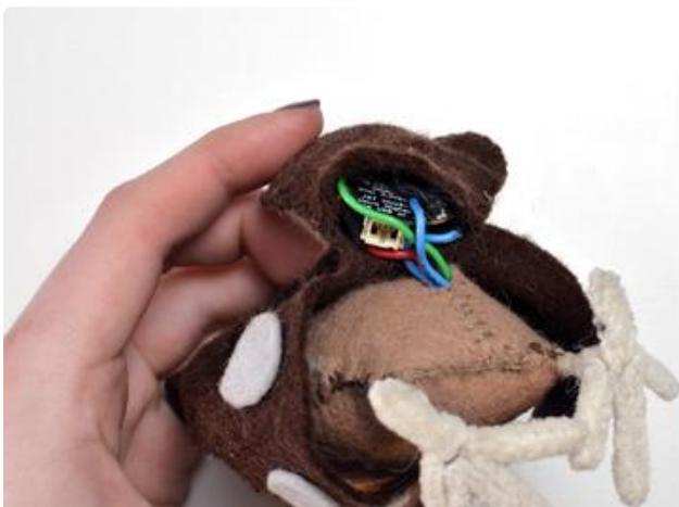
The battery sits inside the cape of the owl, and GEMMA's JST port conveniently faces the opening for convenient disconnection. When the battery runs down you will need to disconnect and remove the battery, and charge it using the MicroLipo charger. (Lithium batteries are not made to be recharged while inside the owl, as the battery may get hot. So that's why you need to remove to recharge). Also the GEMMA v1, v2 and M0 do not support recharging Lithium cells.
