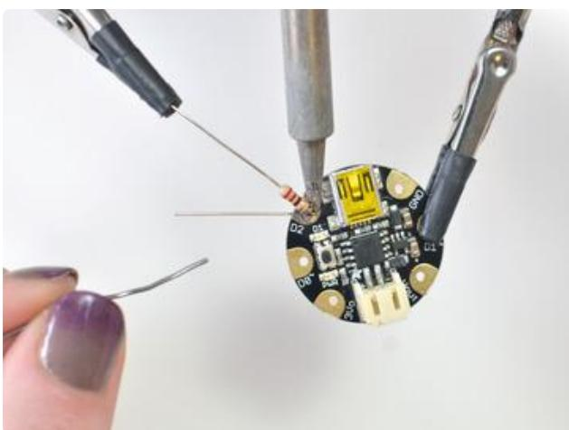
Insert one of the legs of the 220 ohm resistor into the pin marked D2 on GEMMA.
