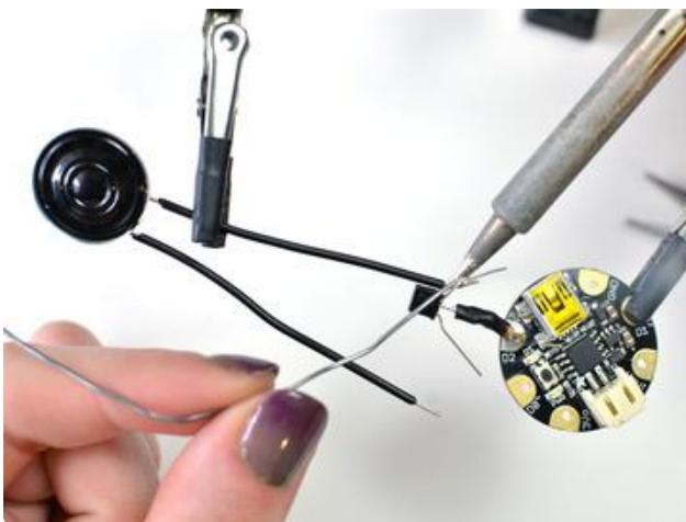
Twist the wires together and solder.
