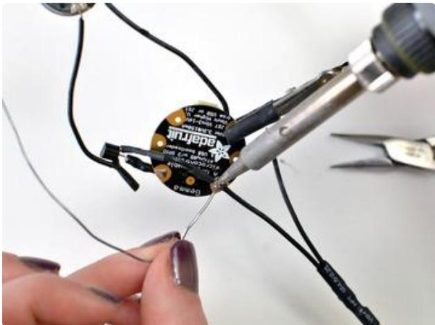
The tilt ball switch has two leads. Solder one lead to D0 on GEMMA and the other lead to GND on GEMMA.
