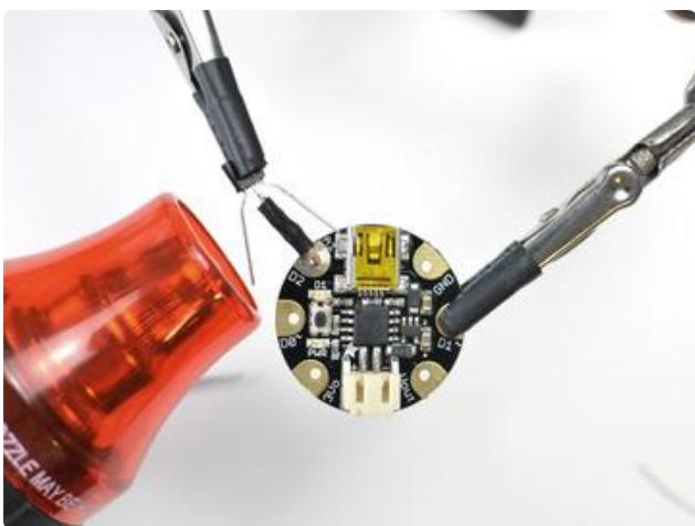
Don't forget heat shrink tubing! Cut a small piece of the medium size and place it over the resistor.
