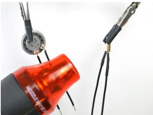
Slide a piece of the smallest diameter heat shrink tubing over each leg of the tilt ball switch to insulate the wires and solder connections.
