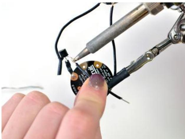
Cut the wire to reach to GND on GEMMA, strip a bit of insulation off the end and solder the end to GND on GEMMA.
