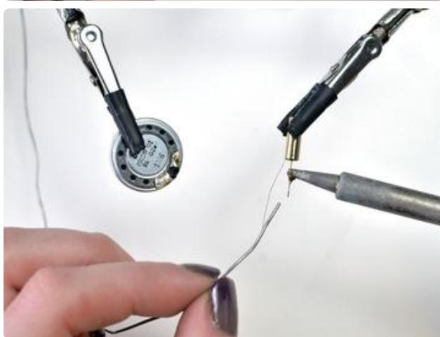
Apply a small amount of solder to the heated pad to tin it. This will make it easier to attach a wire in the next step.
