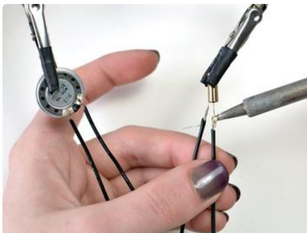
Repeat to solder wires to the the other speaker pad and both legs of the tilt ball switch.
