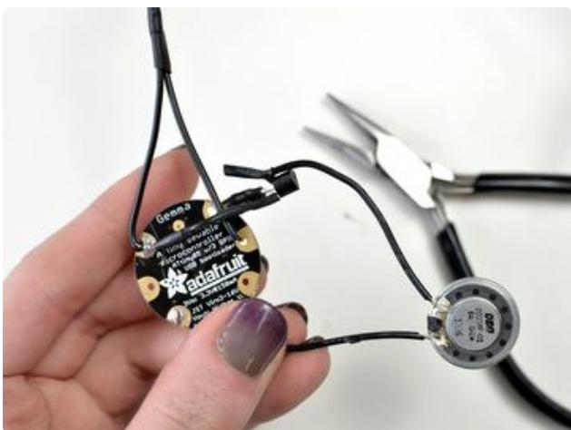
Solder both of these wires to the pad of the circuit board together.
