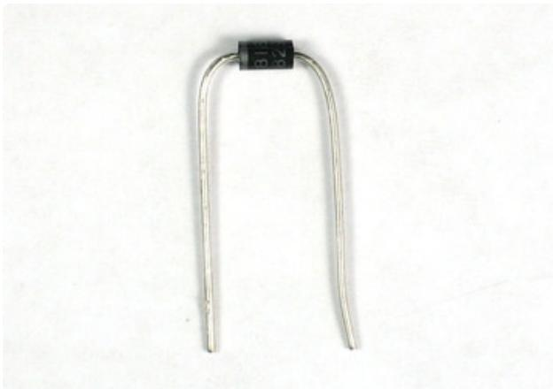
Next we will solder in the 1N5818 protection diode. Diodes only conduct electricity in one direction. This means we can use them to protect our circuitry from negative voltages - a top killer of electronics!
