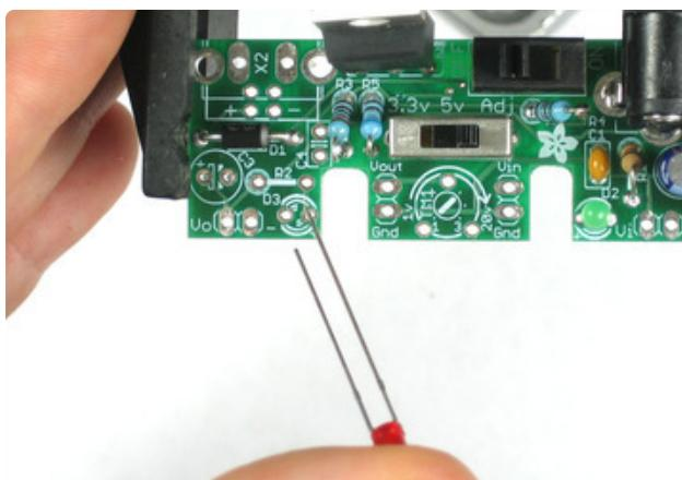
Now we need a way to select which resistor is connected to the regulator. For that we use a 3-way switch. The switch can only go in one way.
