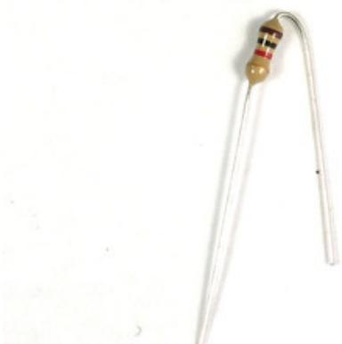
We're going to solder one of the 1.0K resistors in next. The resistors should be bent over 180 like shown. Note that resistors are 'non-polarized' so you can put them in 'either way' - they work the same forwards or backwards.
