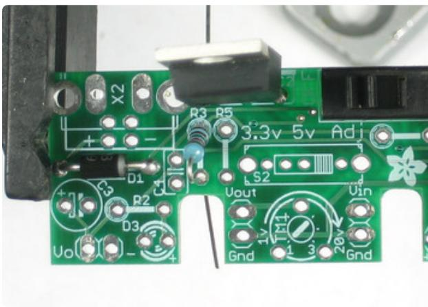
The regulator uses resistors to set the adjustable output voltages. We'll now solder those in.
