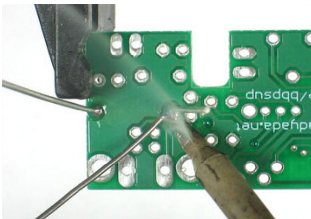
Now solder both wires to the PCB.
