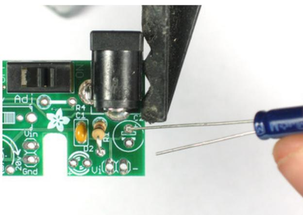
Electrolytic capacitors are **polarized** that means they must go in the right way or they will make your kit not work! See how one leg of the capacitor is longer? That is the positive (+) lead. Make sure that lead goes into the pad marked with a +. See the image left for details.
