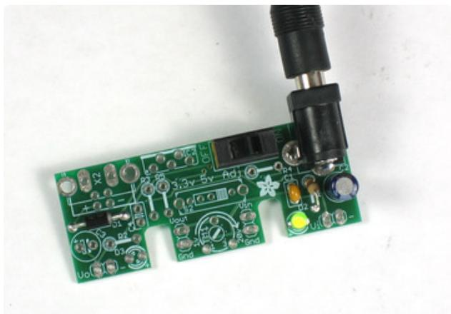
Plug in a DC power supply, center positive. Switch the power switch to the ON position. You should see the green LED light up.
