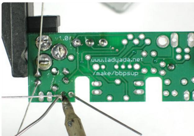
Bend the leads out so the parts sit flat against the PCB.
