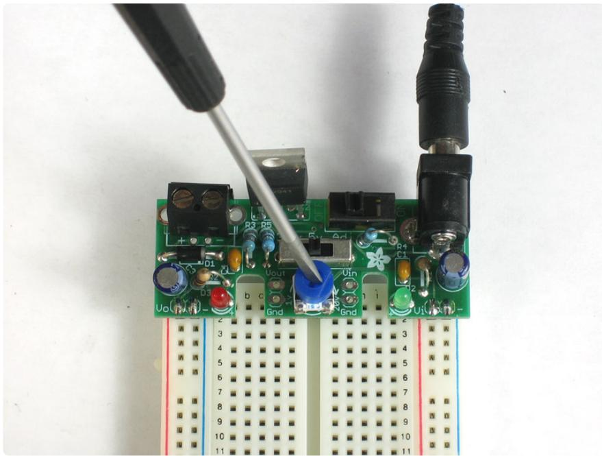
Once you set the pot, the output voltage is not dependent on the input voltage. That is, if you dial in 6V and you switch from a 9V to 12V supply, the output will stay at 6V.
