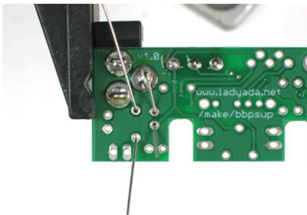
The resistor sets the brightness of the 'high voltage' indicator LED. The 0.1uF capacitor provides high frequency filtration to make the power supply cleaner.
