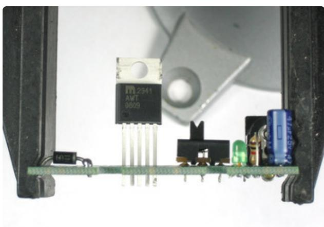
Now we will solder in the heart of the kit, the MIC2941 adjustable voltage regulator. The regulator must be placed correctly to work. Make sure that the big silver tab is at the edge of the PCB (theres a thick white line on the silkscreen to indicate it).
