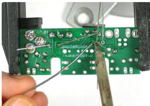
Solder and clip the three resistors.
