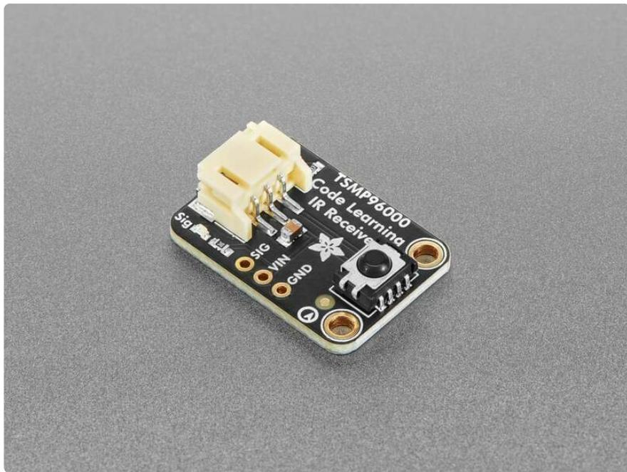
Each STEMMA board is a fully assembled and tested PCB, but no cable. No soldering is required to use it, but you will need to pick up [a 2mm pitch, 3-pin STEMMA JST PH cable](https://adafru.it/18cS) (<https://adafru.it/18cS>). Alternatively, if you do want to solder, there's a 0.1" spaced header for power/ground/signal.
