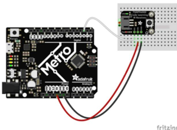
Board 5V to breakout VIN (red wire)
