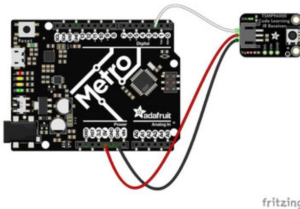
Board 5V to breakout JST PH V+ (red wire)
