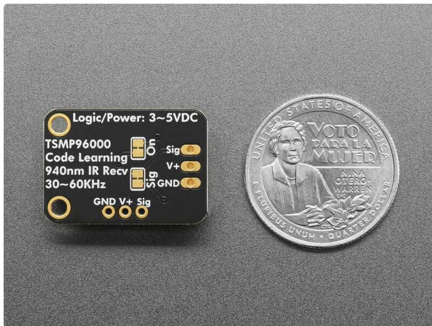
This board will work nicely for advanced IR remote receiving projects, because you don't get the demodulated output it's not good for most IR decoding firmware - make sure you've got code specifically designed for "code learning"! With mounting holes and a cable, it's easy to mount in enclosures and on devices. Using a 2mm pitch STEMMA JST PH cable with headers or alligator clips on the end, you can easily wire this board without any soldering.
