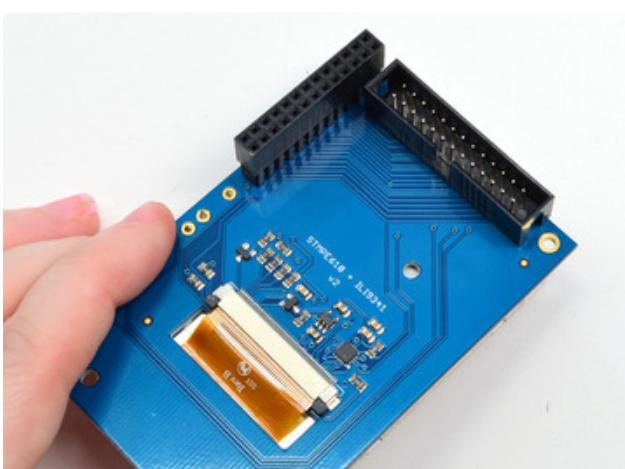
If you want to attach an Adafruit Cobbler or similar, you can solder in the optional 2x13 IDC on the **bottom** of the screen as shown here. This will keep the top side clean and flat. Solder in all 26 pins
