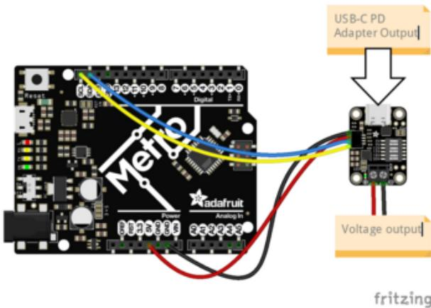
USB C PD power supply to breakout USB C port
