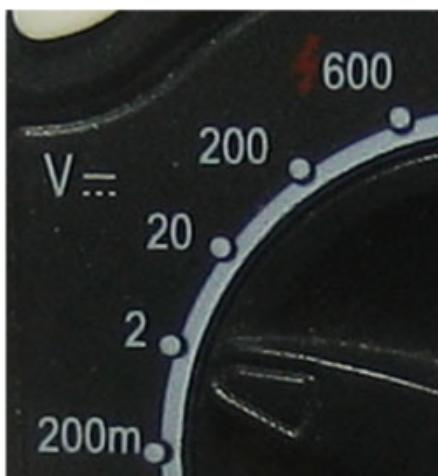
For this example, it's best to test with the output from the breakout connected to a multimeter in DC voltage mode. DC voltage mode is labeled with a V and two lines, one dashed and one solid. [For information on using a multimeter, check out this guide.](https://adafru.it/192A) (<https://adafru.it/192A>)
