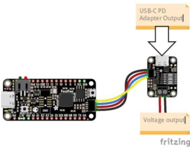
USB C PD power supply to breakout USB C port
