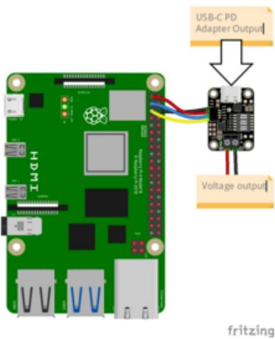
USB C PD power supply to breakout USB C port
