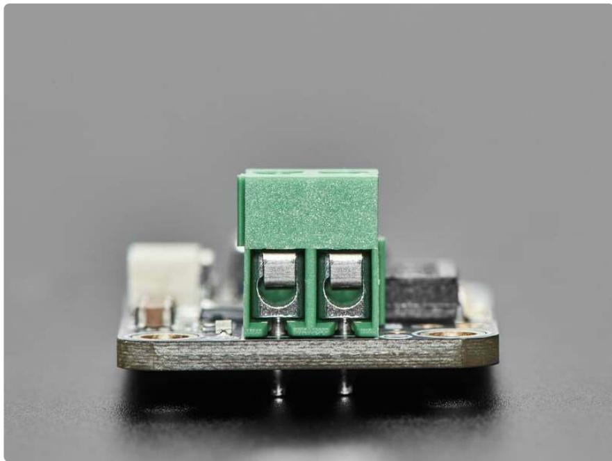
This breakout will be handy for projects where you need a lot more than 5V @ 2A power: this adapter can give up to 20V at 5A - yes you can get 100W over USB C! - and you could buck that down to get a ton of current at 5V or 12V if that's needed. Or use it to convert a DC or battery-powered device into a USB C powered one!
