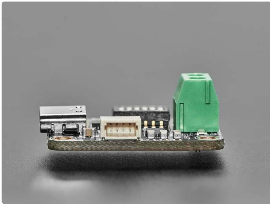
I2C-configured usage is also available via a Stemma QT port. Use the [Arduino library and example code](#) (<https://adafru.it/192c>) to query the USB Type C PD source for available voltages and currents and select the desired voltage dynamically. When configuring over I2C, the jumper settings are used on startup until the I2C commands come over.
