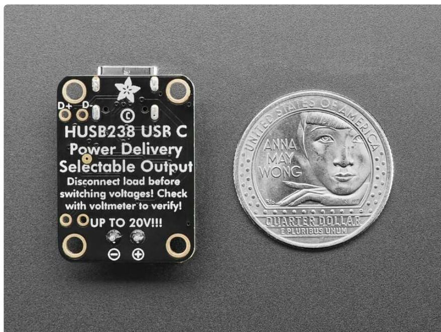
It's perfect for USB Type C wall adapters providing multiple voltages. The standard offerings are 5V, 9V, 12V, 15V, 18V, and 20V. This HUSB238 breakout plugs into the USB C cable and negotiates the PD request and commands over the CC lines. For example, we can ask what voltages are available and pick the highest. Or if you need a specific voltage, it will select that one.
