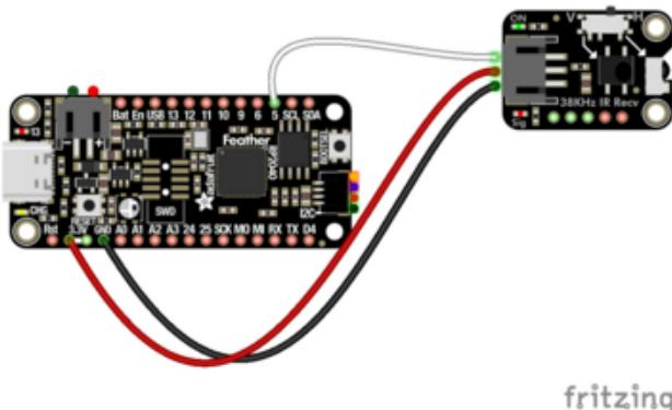
Board 3V to receiver JST PH V+ (red wire)
