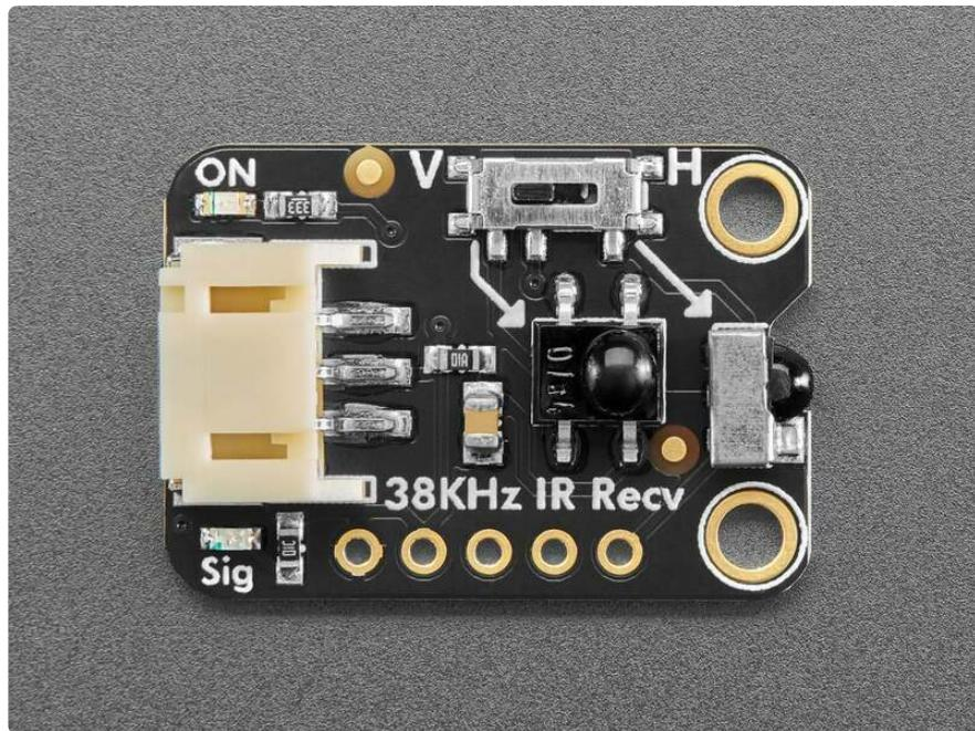
We found plenty of 38KHz receiver sensors that would work nicely on this breakout board - but when it came to choosing one that was vertical or horizontal we just couldn't make up our mind...so why not both? We've placed one on the end and one in the middle, and a slide switch to select which one you want to read the signal from.
