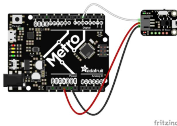
Board 5V to receiver JST PH V+ (red wire)
