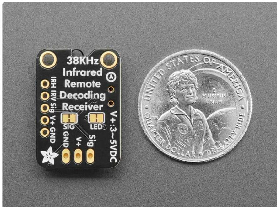
Usage is simple: Power the board by connecting V+ and ground to 3 to 5VDC, point a 38KHz remote control at the sensors and press some buttons. The demodulated IR
