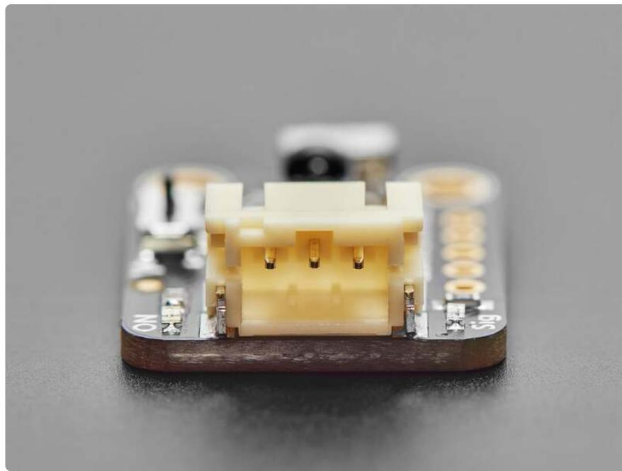
This board will work nicely for a variety of IR remote receiving projects, and with mounting holes and a cable, a lot easier to mount in enclosures and on devices. Using a 2mm pitch STEMMA JST PH cable with headers or alligator clips on the end, you can easily wire this board without any soldering.
