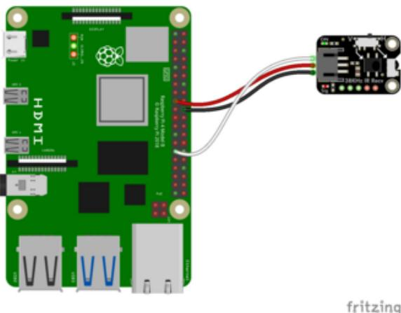
Pi 3V to receiver JST PH V+ (red wire)
