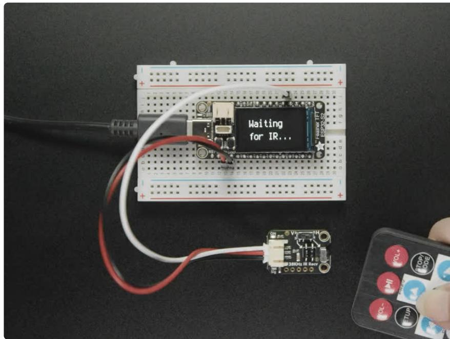
A year ago we designed a high-current-output [Infrared Transmitter STEMMA](http://adafru.it/5639) (<http://adafru.it/5639>) which makes it easy to create high-powered IR LED blasters. Now we've sat down to design the other side, the super sensitive wide-range **Adafruit Infrared IR Remote Receiver** with two selectable IR receiver chips.
