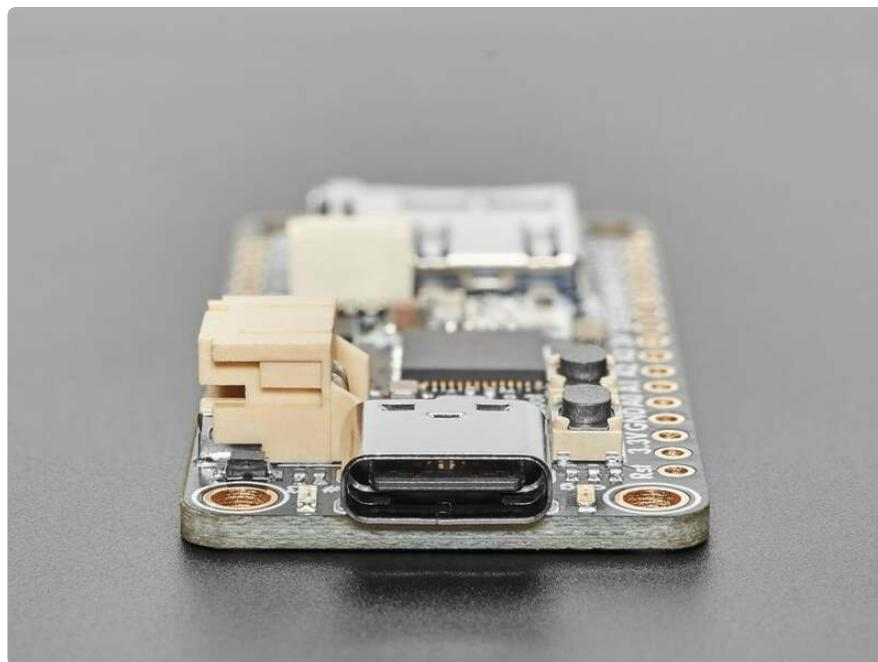
To make it easy to use for portable projects, we added a connector for any of our 3.7V Lithium polymer batteries and built-in battery charging. You don't need a battery, it will run just fine straight from the USB Type C connector. But, if you do have a battery, you
