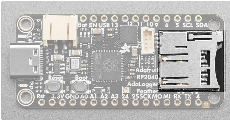
The star of the RP2040 AdaLogger is the microSD card slot for adding as much storage as you could possibly want for reading or writing. It is connected to one of the two available SPI ports (SPI0) on the Feather with an optional card detect line that can be connected to GPIO15. For advanced hackers who want to use 4-bit SDIO, we connect DAT1 and DAT2 to GPIO21 and GPIO22 - note we do not have Arduino or CircuitPython code for this mode.
