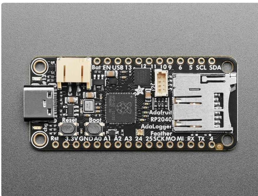
The RP2040 Adalogger is the same size and shape as a Feather and is intended to make your next data logging or data reading project super easy. Micro SD card socket wired for SPI or SDIO? Yes! STEMMA QT / Qwiic connector for fast I2C? Of course!
