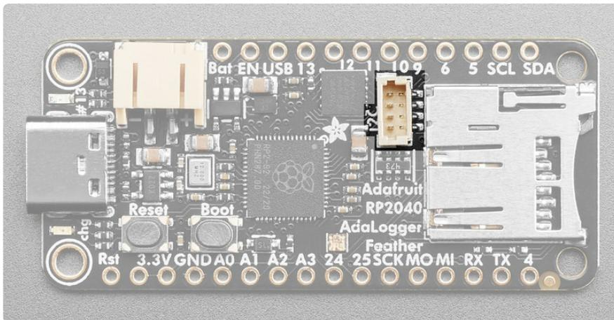
In the middle of the board, to the left of the microSD card slot, is the **STEMMA QT connector**! This means you can connect up [all sorts of I2C sensors and breakouts](https://adafru.it/18fV) (<https://adafru.it/18fV>), no soldering required! This connector uses the SCL and SDA pins for I2C, which end up being the RP2040's I2C1 peripheral. In CircuitPython, you can initialize the STEMMA connector with `board.STEMMA_I2C()` (as well as with `board.SCL` `board.SDA`). In Arduino it is `Wire`.
