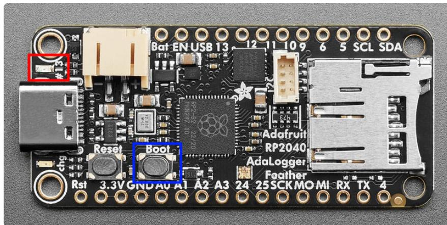
You'll use the Boot button, labeled **Boot** on the board silk, to turn on the build-in LED, labeled **#13** on the board silk.
