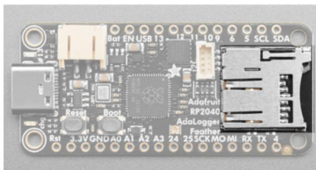
The **MicroSD card slot** is located at the end of the board, directly behind the STEMMA QT port.
