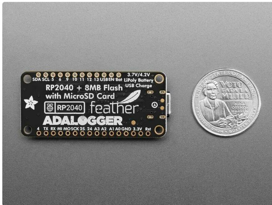
At the Feather's heart is an RP2040 chip, clocked at 133 MHz and at 3.3V logic, the same one used in the [Raspberry Pi Pico](http://adafru.it/4864) (<http://adafru.it/4864>). This chip has a whopping 8MB of onboard QSPI FLASH and 264K of RAM! This makes it great for buffering and processing data before writing it to the SD card.
