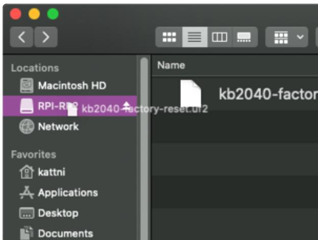
Drag the **factory-reset.uf2** file to the **RPI-RP2** drive.
