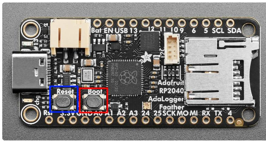
To enter the bootloader, hold down the **BOOT/BOOTSEL** button (highlighted in red above), and while continuing to hold it (don't let go!), press and release the **reset button** (highlighted in red or blue above). **Continue to hold the BOOT/BOOTSEL button until the RPI-RP2 drive appears!**
