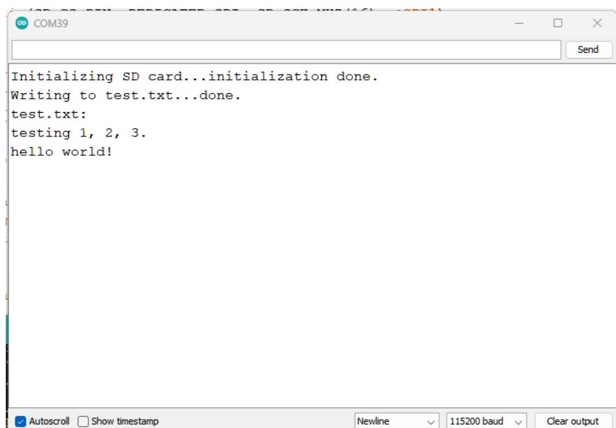
Upload the sketch to your board and open up the Serial Monitor (**Tools** → **Serial Monitor**) at 115200 baud. A test text file will be created and written to on the SD card. Then, the text file will be read back with its contents printed to the Serial Monitor.
