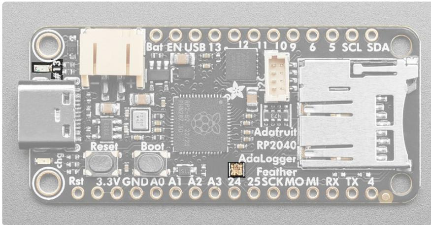
Above the silkscreen label for pin 24 is the status **NeoPixel LED**. It is connected to **GPIO17**. In CircuitPython, the NeoPixel is available at `board.NEOPIXEL` and the library for it is available in [the bundle](https://adafru.it/ENC) (<https://adafru.it/ENC>). In Arduino, it is accessible at `PIN_NEOPIXEL`. The NeoPixel is powered by the 3.3V power supply but that hasn't shown to make a big difference in brightness or color. In CircuitPython, the LED is used to indicate the runtime status.
