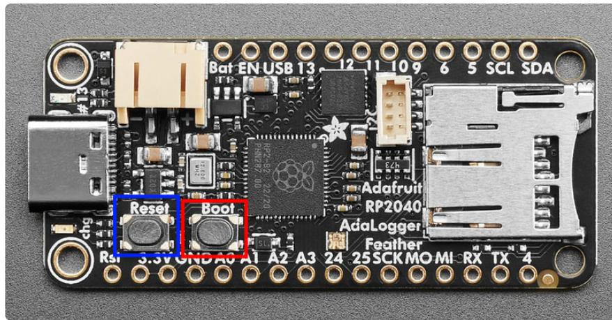
To enter the bootloader, hold down the **Boot button**, and while continuing to hold it (don't let go!), press and release the **reset button**. **Continue to hold the Boot button until the RPI-RP2 drive appears!**
