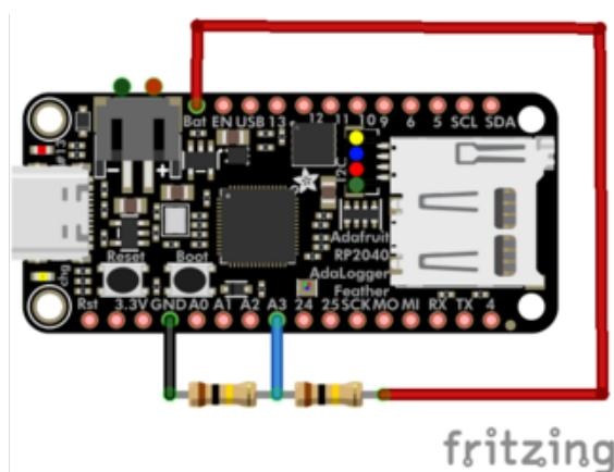
The two 100KΩ resistors are connected in series. One end goes to the **BAT** pin, other end to **GND**, and then the center point between the two resistors goes to any analog pin you'd like to use (**A0** through **A3**). The diagram shows **A3**.
