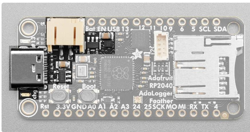
The above shows the **USB C connector** (left center), the **LiPoly JST connector** (top left), as well as the changeover diode (to the right of the JST jack), the 3.3V regulators (to the left of the JST connector and the **USB C** connector) and the charging circuitry (below the JST connector).
