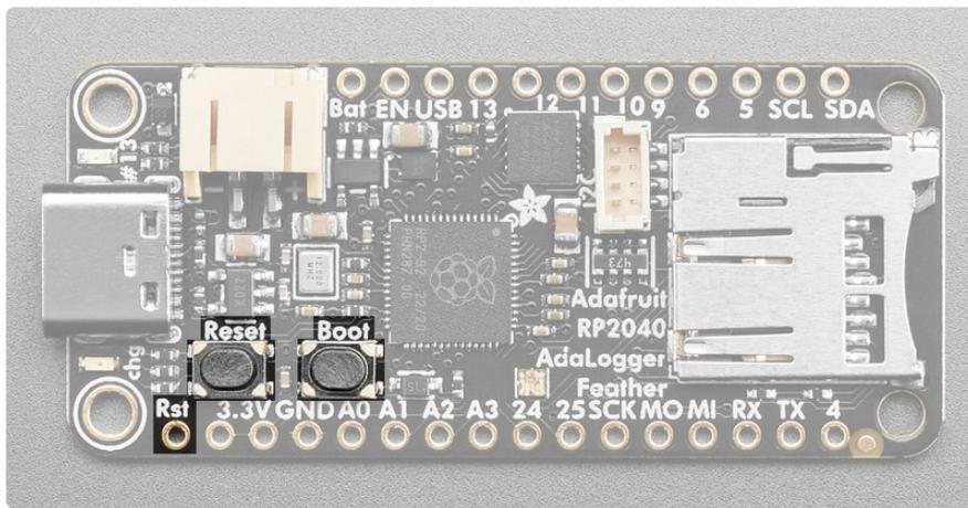
The **Boot button** is the button on the right, located on **GPIO7**. It is available as `board.BUTTON` in CircuitPython and `PIN_BUTTON` in Arduino. It is also used to enter the bootloader. To enter the bootloader, press and hold **Boot** and then power up the board (either by plugging it into USB or pressing Reset). The bootloader is used to install/update CircuitPython.
