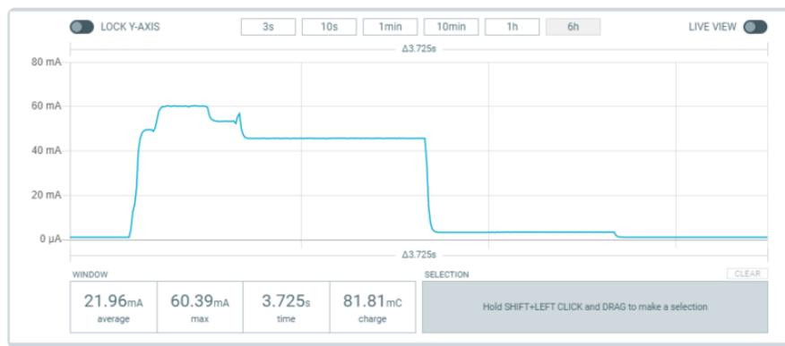
The big pulse is normal mode, you can see the ESP32 booting up, loading code, and then pausing 1 second. Then there's a big drop for one sec to light sleep, and finally one more 1 second pause at deep sleep.
