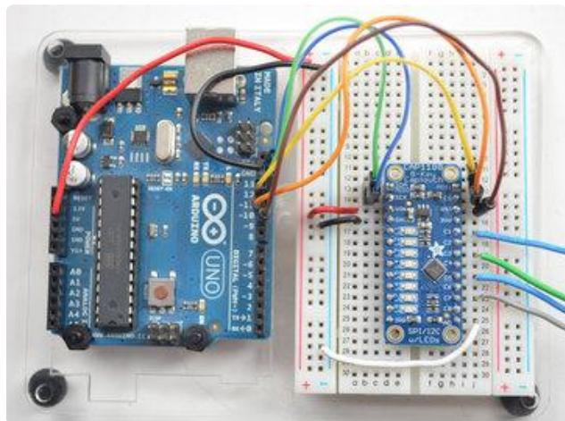
Connect **Vin** to 5V and **GND** to ground, then tie a wire from **AD** to ground as well. Now connect the **SCK**, **MISO**, **MOSI**, **CS** and **RST** pins to your microcontroller. If using an Arduino you can use either the hardware SPI pins which are fixed for each Arduino, or go with software SPI where you select any 5 digital I/O pins
