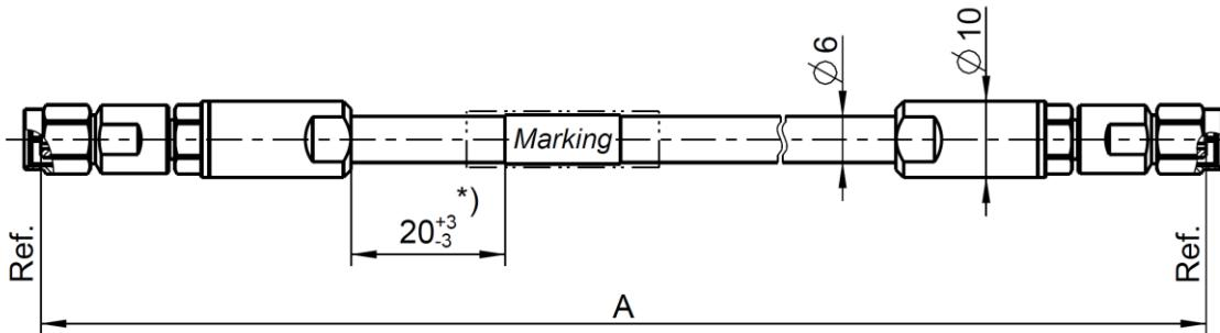
All dimensions are in mm; tolerances: ± 3mm for  $A \leq 300$  mm; ± 1% for  $A > 300$  mm
