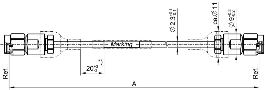
All dimensions are in mm; tolerances:  $\pm 3\text{mm}$  for  $A \leq 300\text{ mm}$ ;  $\pm 1\%$  for  $A > 300\text{ mm}$
