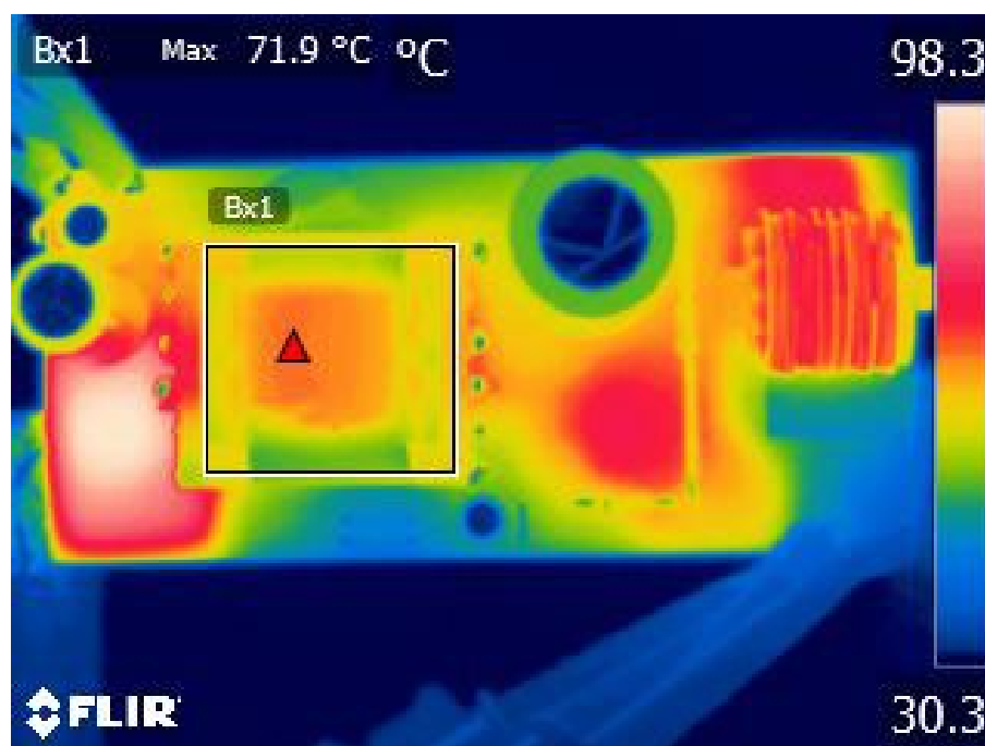
Figure 87 – 85 VAC 60 Hz. Top Side Discrete Component Thermals.
