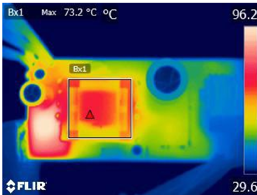
Figure 89 – 265 VAC 50 Hz. Top Side Discrete Component Thermals.
