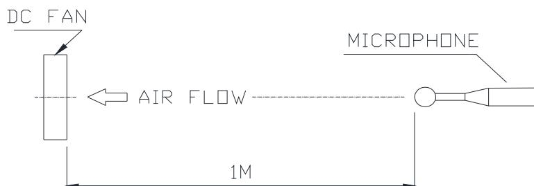
NOISE IS MEASURED AT RATED VOLTAGE IN FREE AIR IN SEMI-ANECHOIC CHAMBER WITH MICROPHONE AT A DISTANCE OF ONE METER FROM THE FAN INTAKE.
