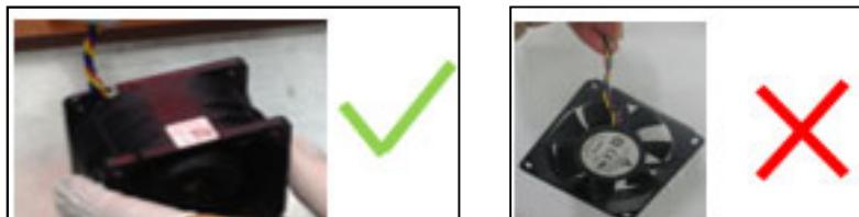
12-1-2. WEARING ELECTROSTATIC GLOVES BEFORE WORKING, MAKE SURE HOUSING ASSAMBLING MECHINE, WORKING TABLE WITH ELECTROSTATIC PROTECTION.
