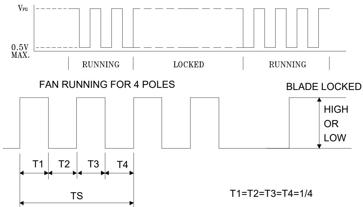
\*VFG IS ALWAYS HIGH OR LOW LEVEL AFTER BLADE LOCKED
