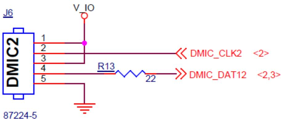
Example DMIC Connector Signal Connections
