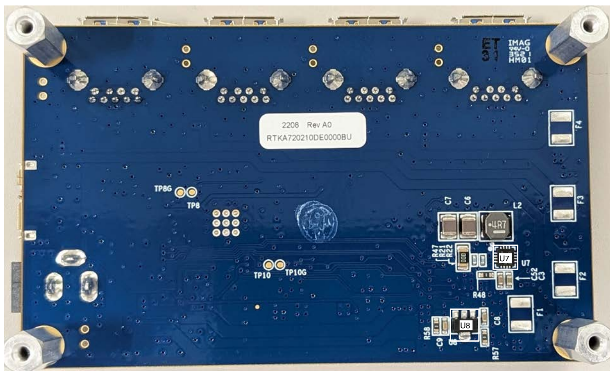
Figure 3. Highlighted Main Parts on the RTKA720210DE0000BU Evaluation Board (Bottom)
