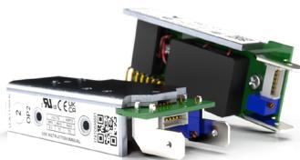
**NEVO+ SERIES****OP2 DATASHEET****Output Module 2: 4.5V-15V, 15A, 150W****OUTPUT MODULE 2 SPECIFICATIONS**
