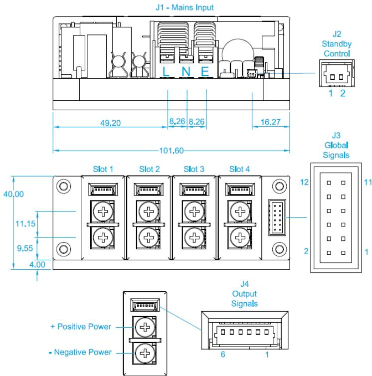
Unless stated otherwise, **All** dimensions are in millimeters and in accordance with DIN2768-1/-2 CLASS C
