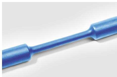
Heat Shrink Tubing, Bulk Reel, 2:1 Shrink Ratio, 1.5", 38.1/19.1 Dia, PO, Blue, 100 ft/reel
