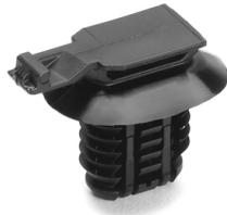
Connector Clip with Oval Fir Tree, 8.0 - 15.0mm Hole Dia, PA66HIRHSUV, Black, 5000/carton
