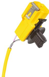
Connector Clip with Oval Fir Tree, 0.6-6.0 mm Panel Thick, 6.2x12.2 mm Hole Dia, PA66HIRHS, Black, 1000/pkg
