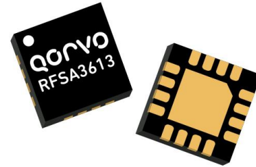
16 Pin 3 x 3 x 0.85mm QFN Package
