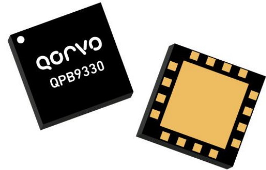
16 Pin 8 mm x 8 mm leadless SMT Package
