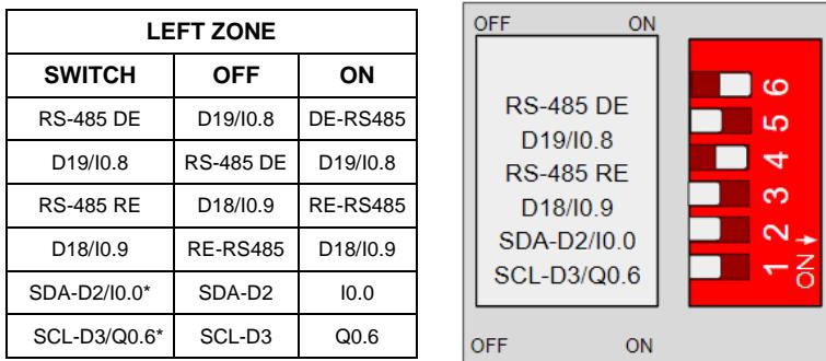
\*I2C switch serigraphy is turned around. It should be: (SDA-D2 , SCL-D3). RX-RS485 should be RE-RS485
