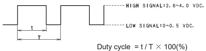
The frequency for control signal of the fan shall be able to accept at 20 kHz-30 kHz.
