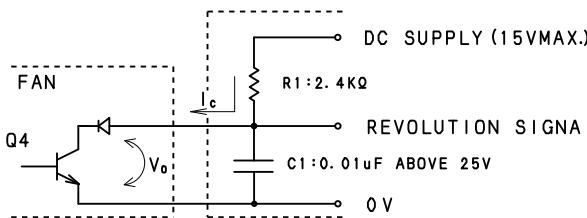
Remark: As for measuring  $V_{OL}$ , it is necessary to put cr low pass filter which is constructed of R1 and C1. The time constant of  $R1 \times C1$  is to be more than 24us such as  $R1=2.4\text{ k}\Omega$   $C1=0.01\text{ }\mu\text{F}$ .
