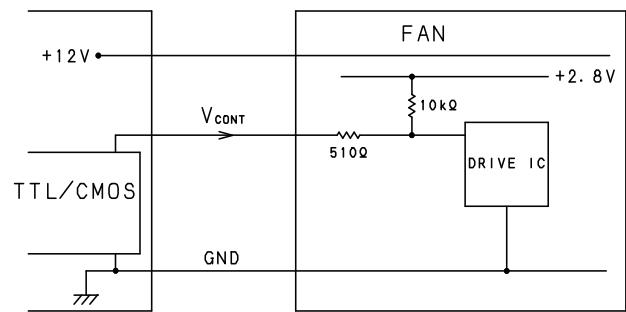
$V_{CONT}$  is above 2.6 V ⋯ Fan should run full speed.
