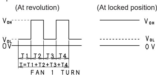
Remark: At locked position, output becomes  $V_{OH}$  OR  $V_{OL}$ .
