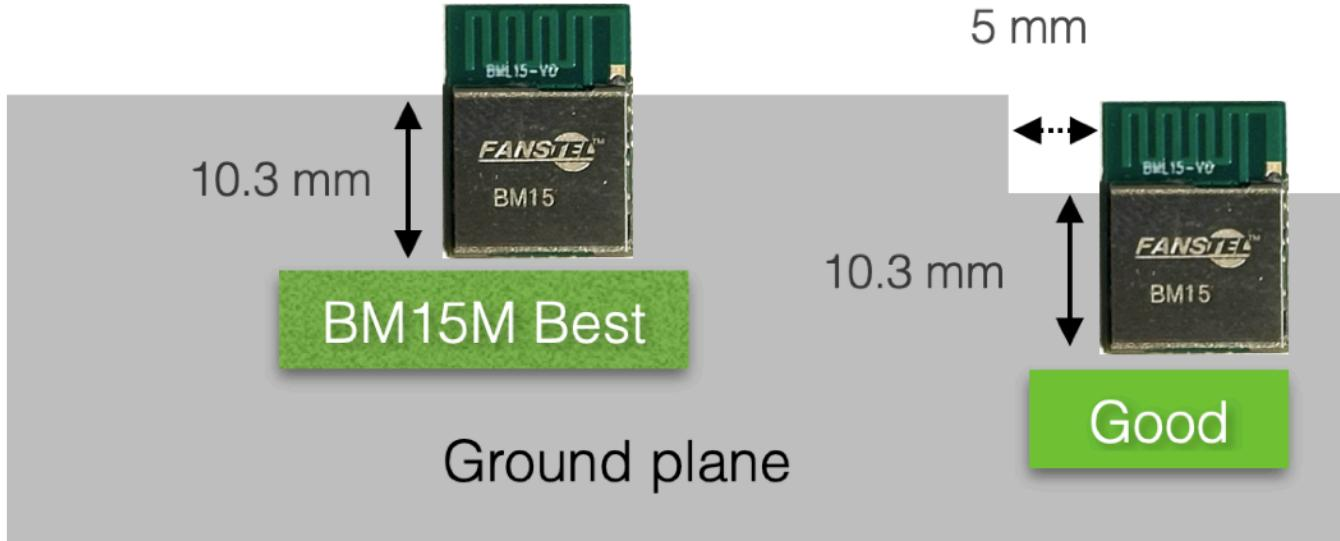
The length of the RFI shield is 10.3 mm. The RFI shield area is the main body of module. The rest of the module is called antenna area.
