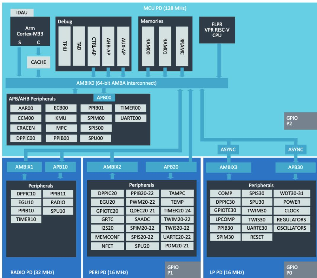
The main processing unit is an ARM Cortex M33 processor running at up to 128 MHz, supported by nonvolatile RRAM and RAM memory. The ARM Cortex M33 has a full set of digital processing (DSP) instructions and a memory protection unit (MPU) for application security. The full-featured single-precision floating-point unit (FPU) supports all single-precision instructions.
