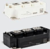
The family of BM 62 mm modules comes in 1.2 kV and 1.7 kV half-bridge topologies that deliver up to 530 A. Material for these modules have been selected to target different operating conditions. Wolfspeed offers THB-80 qualified housing material option to provide additional robustness for applications against harsher environment.
