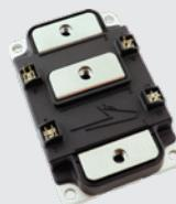
With half the weight and volume of a standard 62 mm module, the XM3 power module maximizes power density while minimizing loop inductance and enabling simple power bussing. The XM3's Silicon Carbide optimized packaging enables 175°C continuous junction operation with a high reliability silicon nitride ( $\text{Si}_3\text{N}_4$ ) power substrate to ensure mechanical robustness under extreme conditions.
