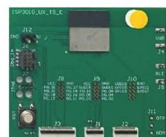
It also offers test points for all IOs and can be used in conjunction with a Nordic Development kit or an external J-Link programmer.
