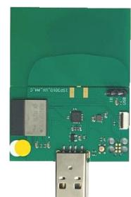
The Tag Board consists of a small PCB integrating an ISP3010 module powered by a coin cell.
