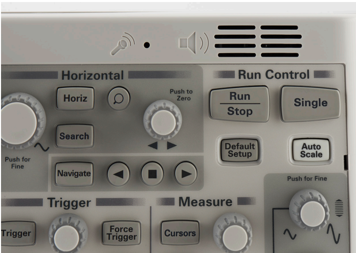
Figure 39. Voice control microphone and speaker.
