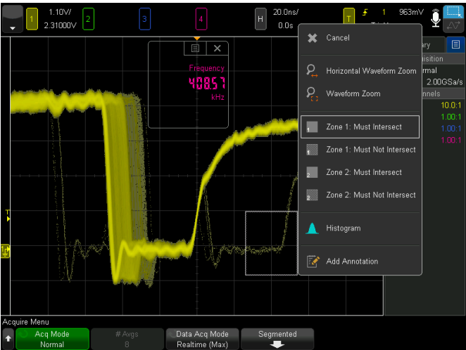
Figure 11. Draw a zone (box) around the anomaly.
