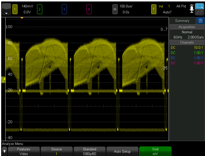
Figure 45. Triggering on a 1080p/60 signal.
