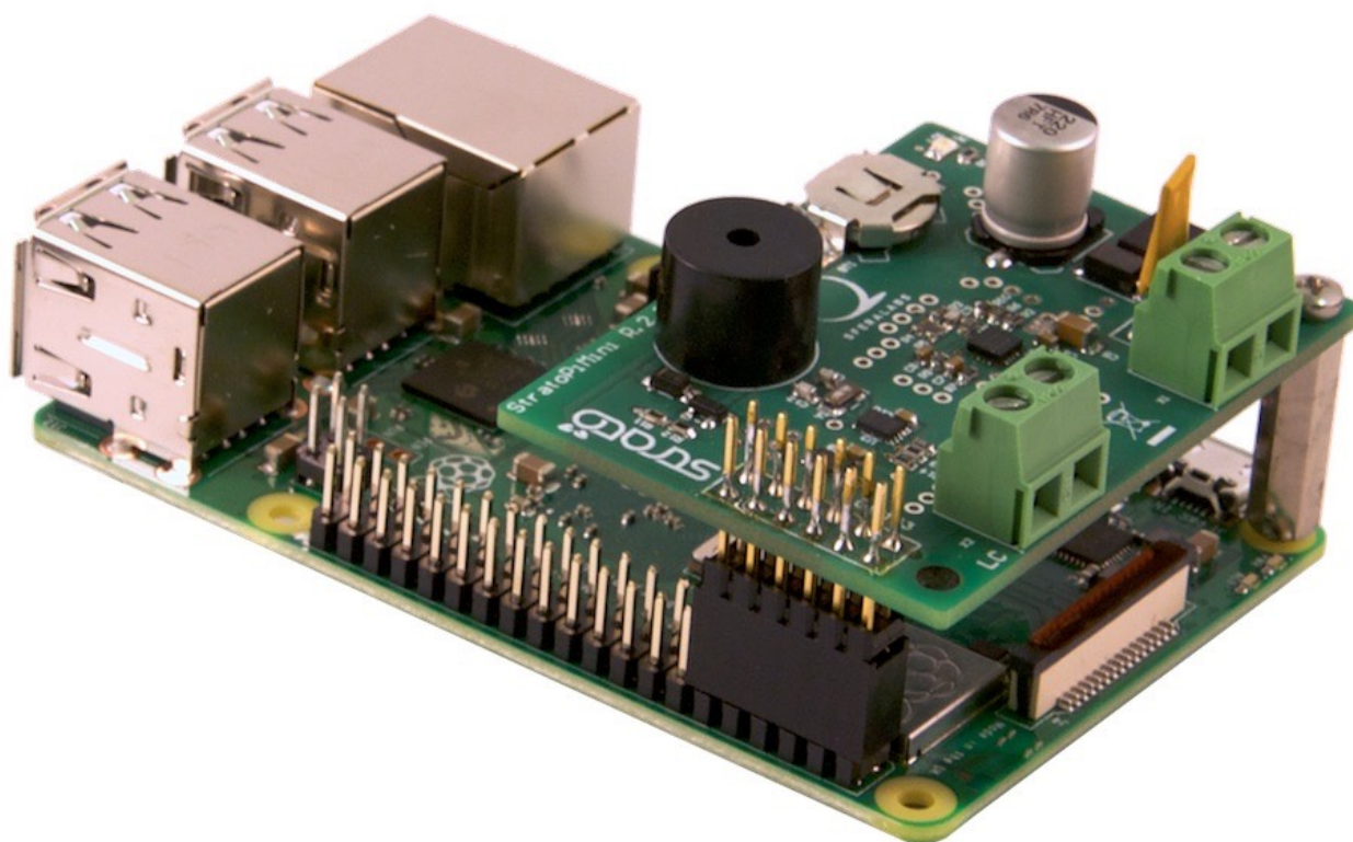
STRATO PI MINI BOARD INSTALLED ON THE RASPBERRY PI
