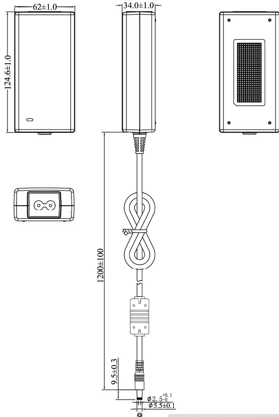
DC Cable: UL1185 16AWG 1200 mm
