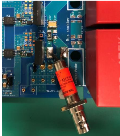
Figure 6.4-1 Measurement method with coaxial shunt resistor
