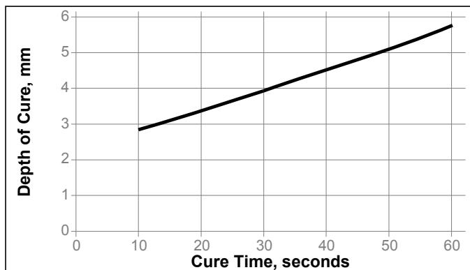
LED Flood Array 405nm, 100 mW/cm<sup>2</sup>, measured @ 405 nm
