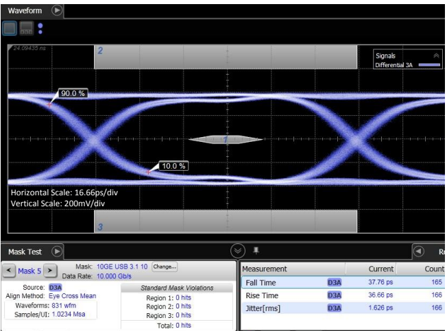
10Gb/s (USB 3.1) Eye Diagram without RClamp3371ZC
