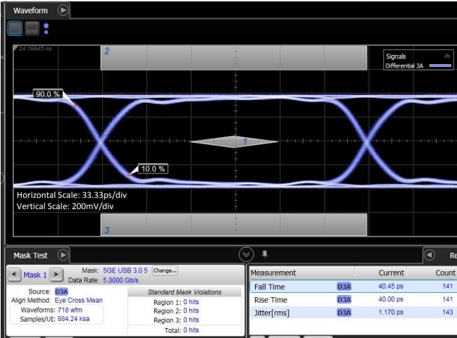
10Gb/s (USB 3.1) Eye Diagram with RClamp3371ZC
