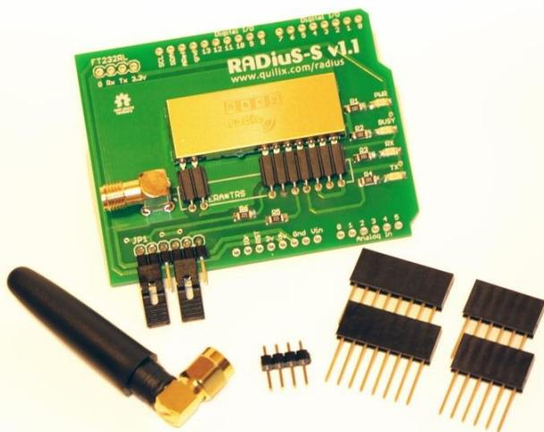
This 'shield' allows Arduino™ boards to communicate wirelessly using proprietary LPRS 'easyRadio' technology operating in the 433MHz or 868MHz (UK & Europe) & 915MHz (US) Industrial Scientific & Medical (ISM) bands.
