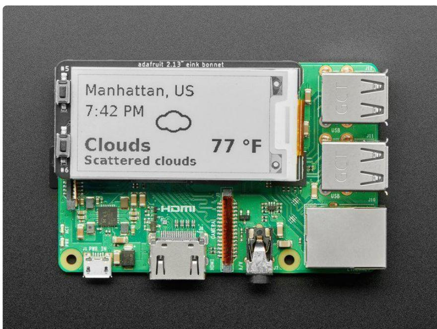
The Adafruit 2.13" Monochrome E-Ink Bonnet for Raspberry Pi snaps onto any modern Raspberry Pi and provides a Python-programmable display with two buttons that can be used to select programs or scroll through options.
