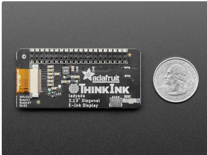
On the bottom, we have a Qwiic/STEMMA QT connector for I2C sensors and devices so you can plug and play any of our STEMMA QT devices (<https://adafru.it/GfR>).
