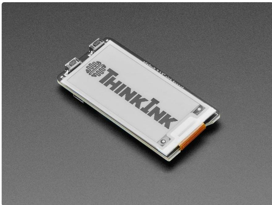
Easy e-paper finally comes to Raspberry Pi, with this bonnet that's designed to make it a breeze to add a 2.13" 250x122 crisp monochromic eInk display. Chances are you've seen one of those new-fangled 'e-readers' like the Kindle or Nook. They have gigantic electronic paper 'static' displays - that means the image stays on the display even when power is completely disconnected. The image is also high contrast and very daylight readable. It really does look just like printed paper!
