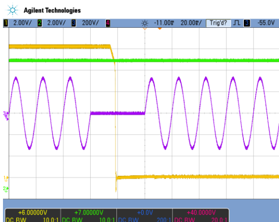
Figure 13. AC drop out 40 ms, full load (20 ms/div) CH1: V1 (2 V/div); CH2: VSB (2 V/div); CH3: Vin (200 V/div)
