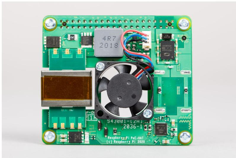
The Raspberry Pi PoE+ HAT is an add-on board for Raspberry Pi computers with PoE pins, including Raspberry Pi 3B+ and Raspberry Pi 4. It is used to power Raspberry Pi via an Ethernet cable, provided that power-sourcing equipment is installed on the Ethernet network. The HAT also includes a fan that will cool the Raspberry Pi processor.
