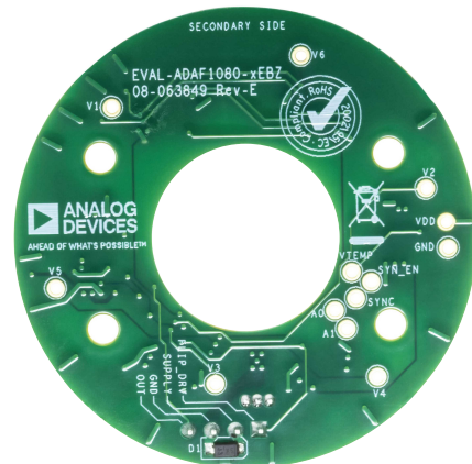
Figure 2. Bottom Side of the EVAL-ADAF1080-6EBZ
