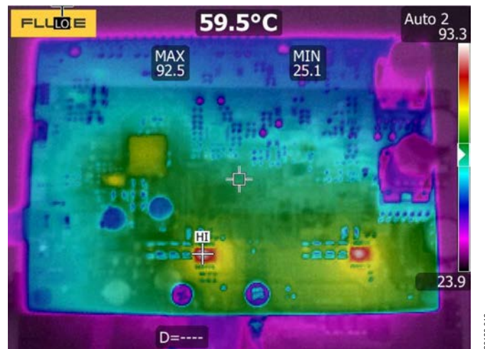
Figure 11. Thermal Image of EVAL-CN0508-RPZ at 30 V Input, 2.75 A Current-Limit Output into 4 \Omega Load
