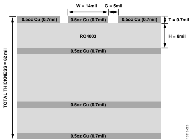
Figure 23. Evaluation Board (Cross Sectional View)
