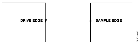
Figure 34. SPI Mode 3 SCLK Edges
