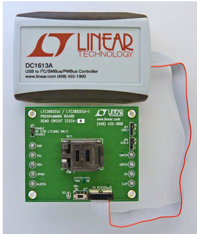
Figure 3. DC1613A Ribbon Cable Installation
