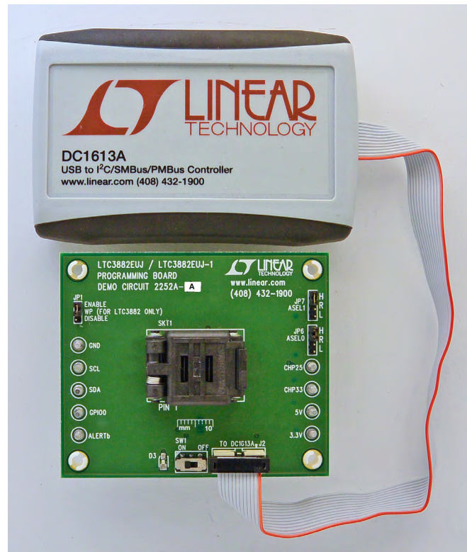
Figure 3. DC1613A Ribbon Cable Installation
