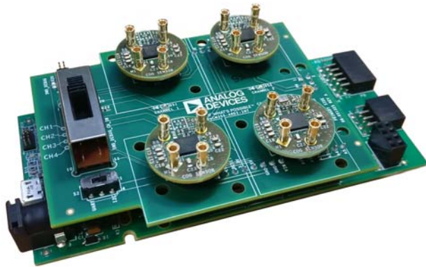
Figure 4. System Setup— EVAL-ADICUP3029 with Four Gas Sensor Boards Connected
