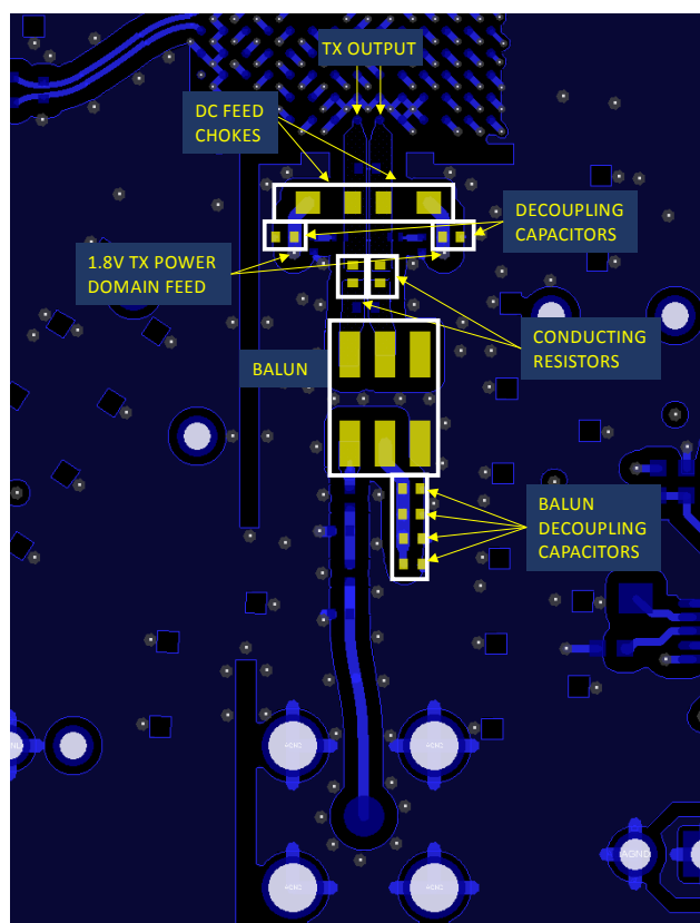
Figure 280. Transmitter DC Chokes and Balun Feed Supply
